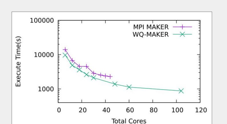
Comparison of execution time using MPI and WQ-MAKER on variable number of cores, evaluating subset of Hummingbird Genome(900MB)
