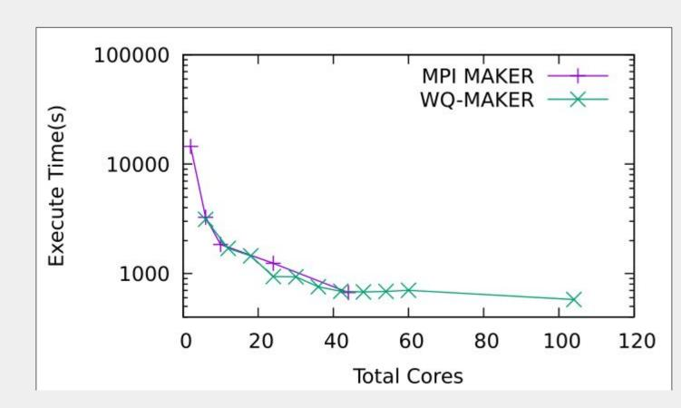
Comparison of execution time using MPI and WQ-MAKER on variable number of cores, evaluating Fungal Genome(41MB)
