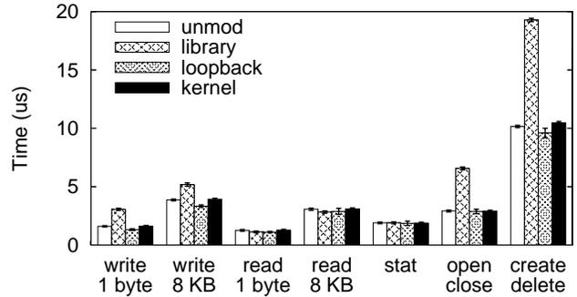
Fig. 7. Latency of I/O Operations
