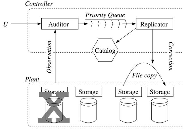
Fig. 2. Replica Control Loop.
