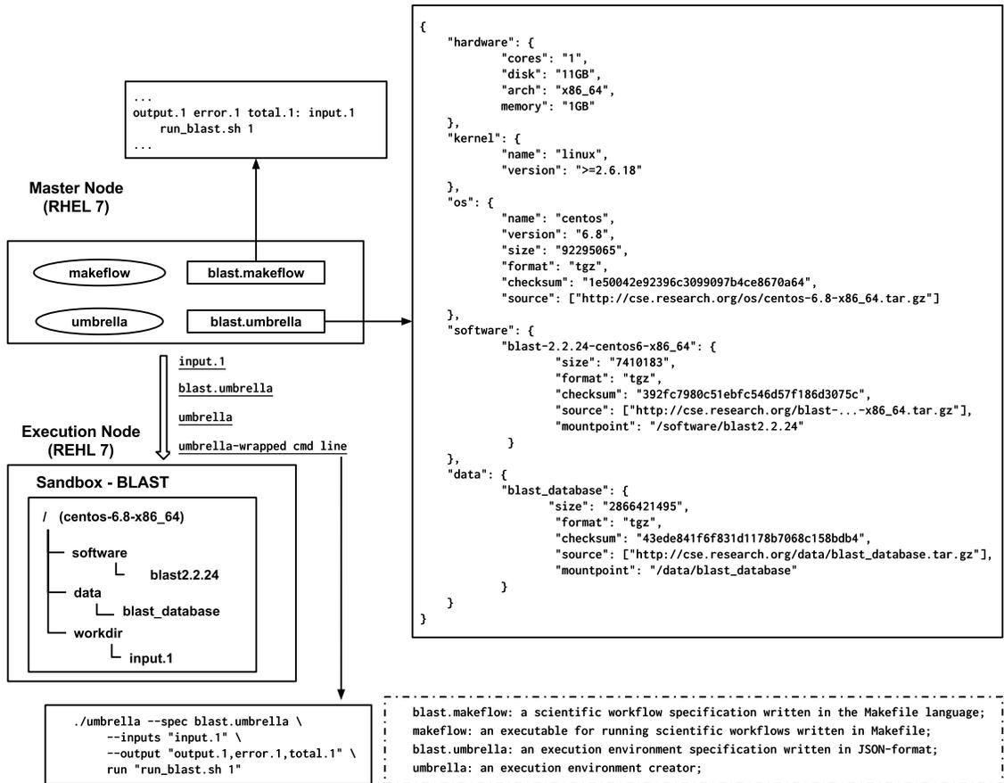
Figure 5.4. Running BLAST with Makeflow and Umbrella
