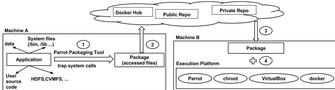
Figure 3.4. Workflow of Creating, Distributing and Deploying Packages
