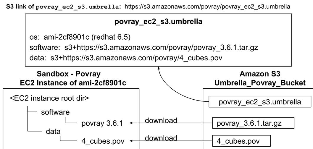
Figure 4.5. Conducting Reproducible Research Using Umbrella - EC2 + S3
