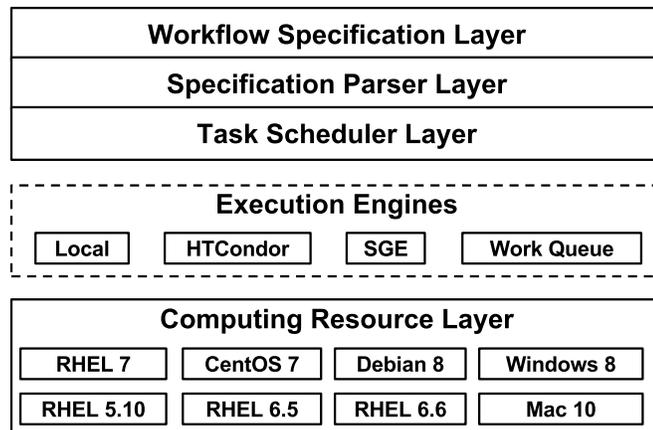
Figure 5.3. Layers of Scientific Workflow Systems
