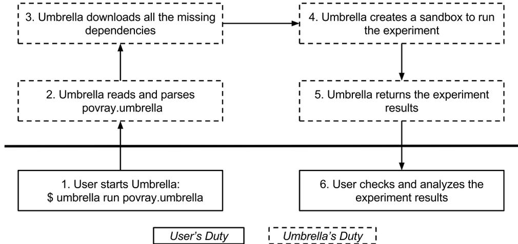
Figure 4.1. Workflow of Umbrella Execution Engine
