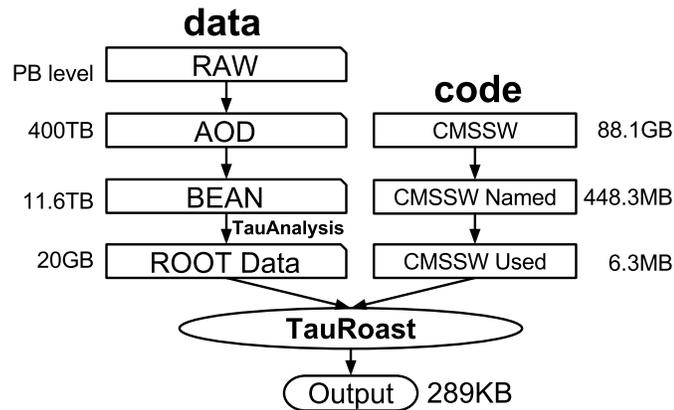
Figure 3.1. Code/Data Inputs to TauRoast and Code/Data Sizes
