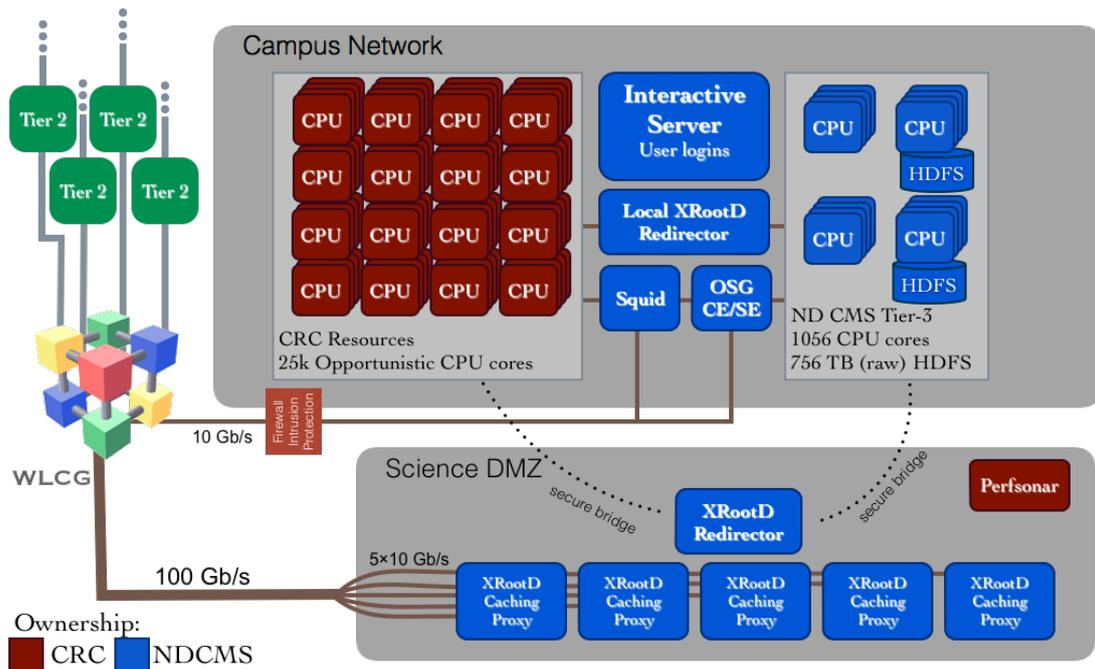
**Figure 1.** This diagram shows the configuration of dedicated ND Tier-3 (labeled NDCMS and shown in blue) and CRC (shown in red) resources used to extend the ND Tier-3 with opportunistic CRC resources. In general, resources from the campus network are unable to access the Science DMZ except by using the the “secure bridge” links as illustrated.
