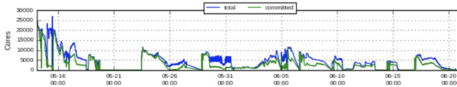
**Figure 4.** Plot showing number of cores used by Lobster, peaking around 25,000 cores. The 25,000 core peak was achieved when the ND CMS team was granted exclusive use of CRC resources during a maintenance downtime. The rest of the plot shows running done during regular CRC operations in competition with other users. Even during these periods, there are times when as many as 10,000 CPU cores can be utilized.
