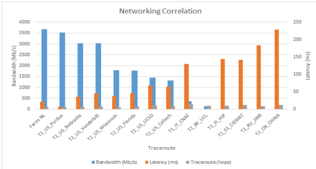
**Figure 2.** Measurements using of bandwidth, latency, and number of hops made using PerfSonar. There is a loose correlation between bandwidth and latency, but there is enough variation from one site to the next to suggest that further debugging of network connections could be beneficial.
