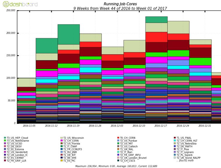
**Figure 6.** This plot shows the number of CPU cores utilized by running jobs at various CMS WLCG sites. The contributions from ND’s Tier-3 site over the period shown are larger than most other Tier-1 and Tier-2 sites. The only Tier-3 site providing comparable CPU resources is the “HEPCloud” site which is an experimental facility operated by Fermi National Laboratory making use of AWS and Google Cloud resources. Note: 61 sites are compressed into the bottom-most contribution in the plot.
