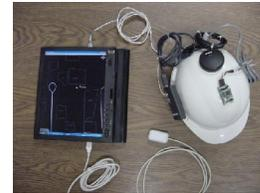
*Figure 1 – The TeamTrak hardware consists of 24 tablet computers, each connected to a pedometer and a sensor helmet mounting GPS, compass, and video camera.*
