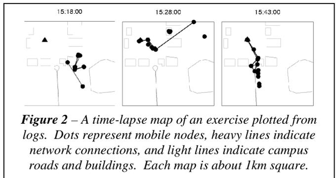
**Figure 2** – A time-lapse map of an exercise plotted from logs. Dots represent mobile nodes, heavy lines indicate network connections, and light lines indicate campus roads and buildings. Each map is about 1km square.
