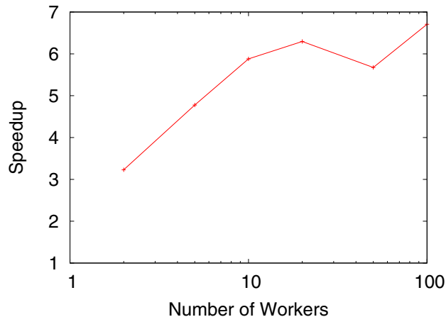
Fig. 2: Speedup of BWA relative to the BWA Tool originally in the Galaxy Toolshed. The results were calculated using S = T_S/T_P , where the sequential time is the runtime for the original tool.
