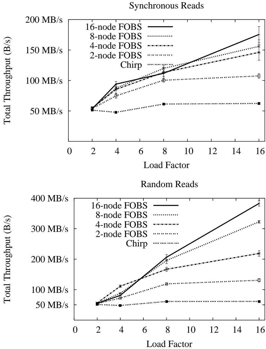
Figure 4.1: Aggregate Filesystem Read Bandwidth Under Load
