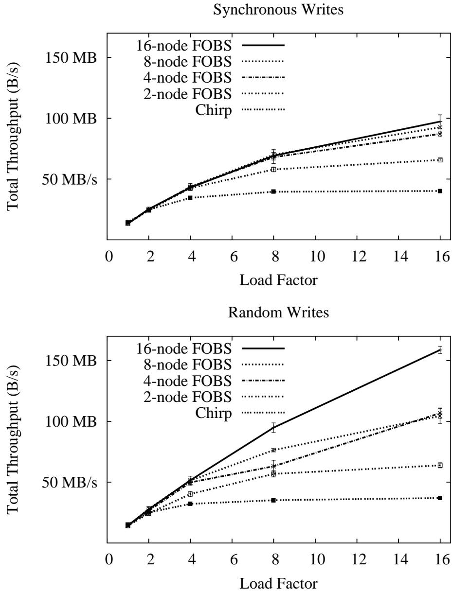
Figure 4.2: Aggregate Filesystem Write Bandwidth Under Load
