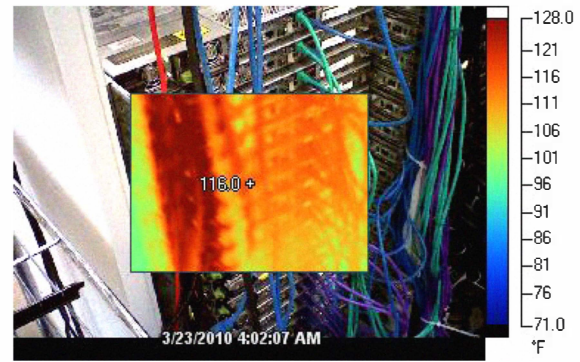
Figure 4. Sample Server Outlet Temperatures via Infrared
