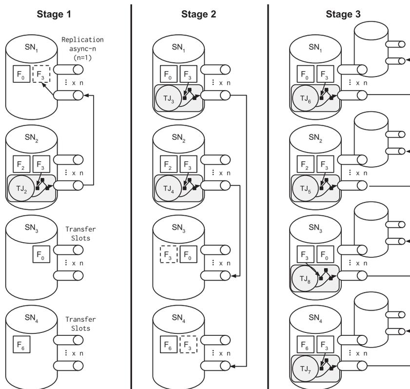
Figure 7. Spanning tree of push transfers. Each push is a transfer job (TJ). One transfer slot per SN ( $n = 1$ ).
