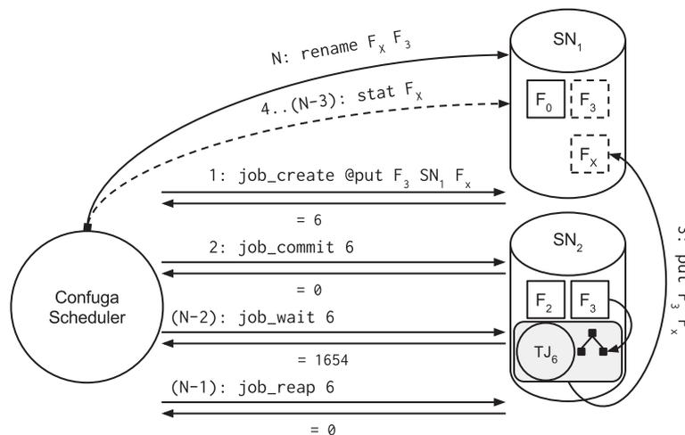
Figure 5. Push transfers are a series of short blocking operations that create a transfer job on the storage node. The transfer job executes asynchronously with the head node. Operations are numbered in order.
