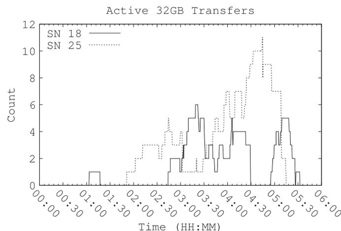
Figure 13. **Workflow C:**  $PT=32$  GB active 32GB pull transfers. This graph shows the groups of pull transfers that are delayed together by disk seeks, resulting in periodic sharp drops in active transfers.
