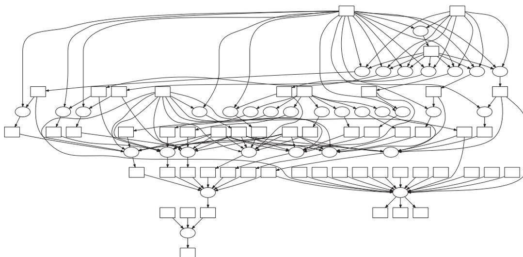
Figure 3. A typical directed acyclic graph-structured workflow. This comes from a bioinformatics workflow using SHRiMP [29]. Here, files are boxes, circles are tasks, and lines indicate dependencies.
