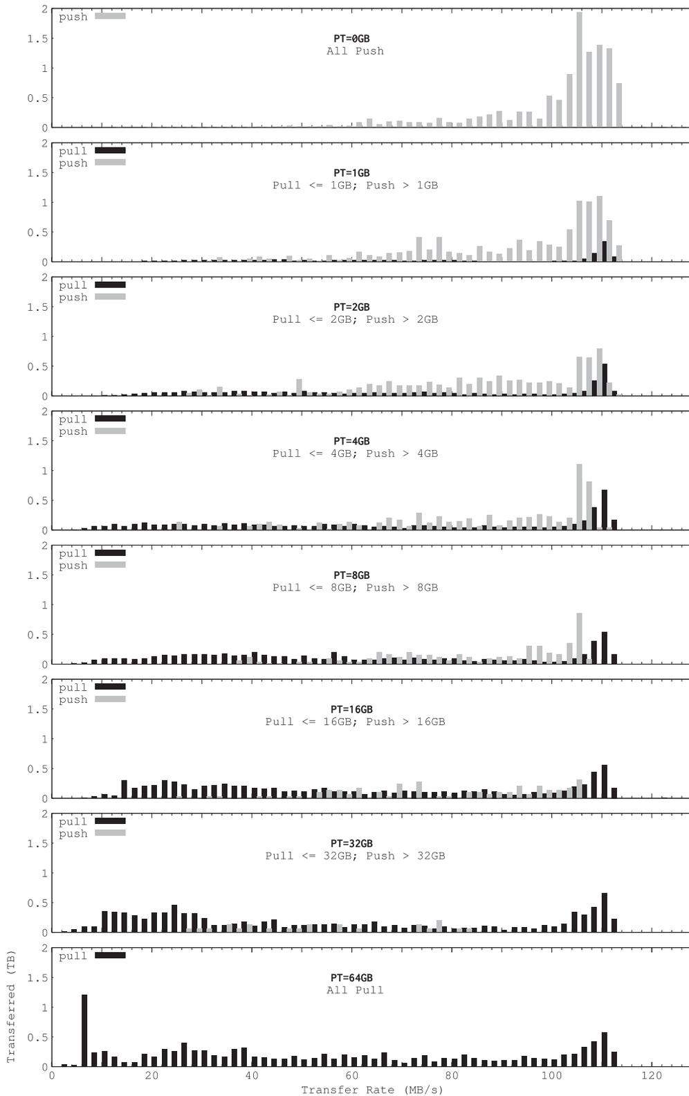
Figure 11. Workflow C: average transfer speed histogram.
